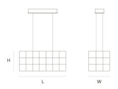
Universe Square is structured but still harmonious. Modular placed E10 light bulbs and tiny metal rods are the only two basic elements of this light fixture. They give the fixture its structure and shape. (see model Cosmos Square for the version with led circuit boards)
